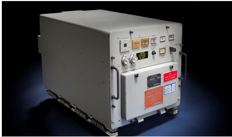
Figure 2: Transit System receivers received navigation signals transmitted by Transit satellites passing overhead and weighed as much as 250 pounds. Credit National Air and Space Museum, Smithsonian Institution
