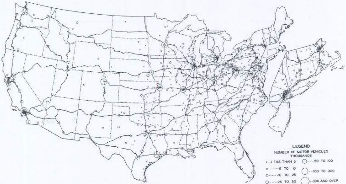
FIGURE 12.—The recommended interregional system in relation to concentrations of motor-vehicle ownership in cities of more than 10,000 population.
