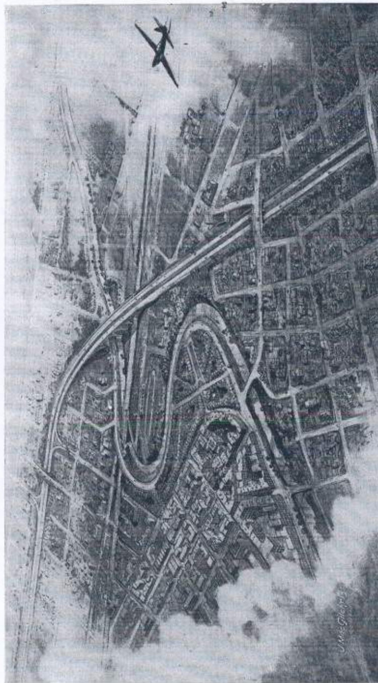
PLATE 30.—A four-lane toll highway in a suburban and urban area, showing relation to existing streets.
