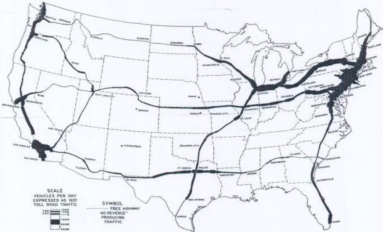
PLATE 11.—Estimated average daily traffic on routes selected for study if operated as toll roads.
