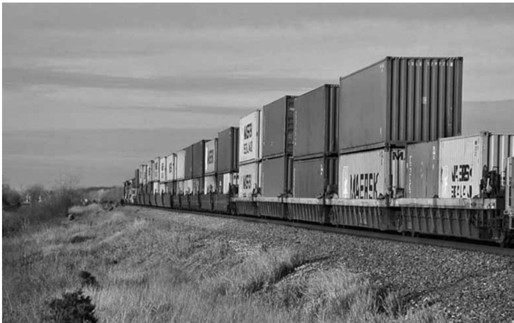
► Figure 11-7 Modern articulated double-stack equipment
