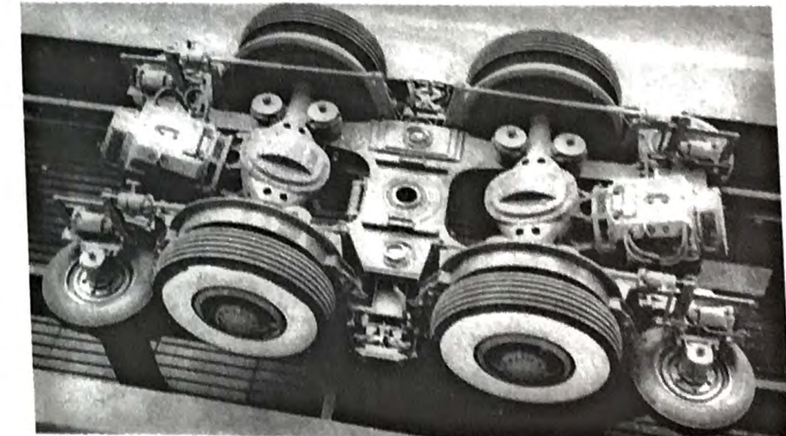
Motor Bogie (Truck) of Pneumatic-Tired Subway Car Developed by Régie Autonome des Transports Parisiens (Paris Metro)
